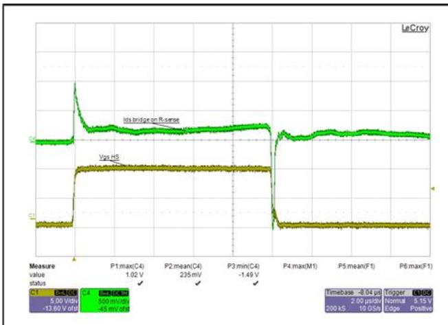
Fig. 7. Short circuit test for STL285N4F7AG
