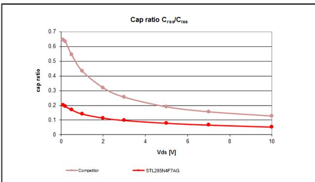
Fig. 2. Measured capacitance ratio  $C_{rss}/C_{iss}$  for STL285N4F7AG vs competition
