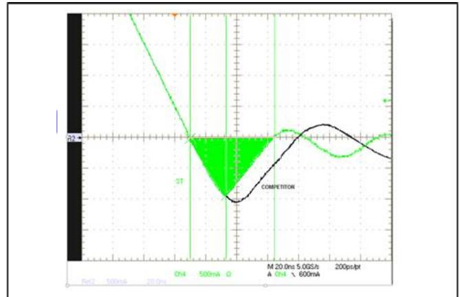
Fig. 3. Measured body-drain diode performance of STL285N4F7AG vs competition
