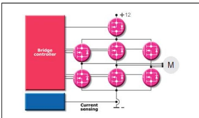
Fig. 1. Servo unit topology for both EPS and EPB systems
